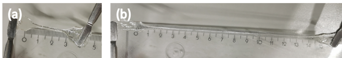
Figure 2. Optical images of PEGMEA-co-PEG-DA-co-AN while stretching to 400% (a, b).
