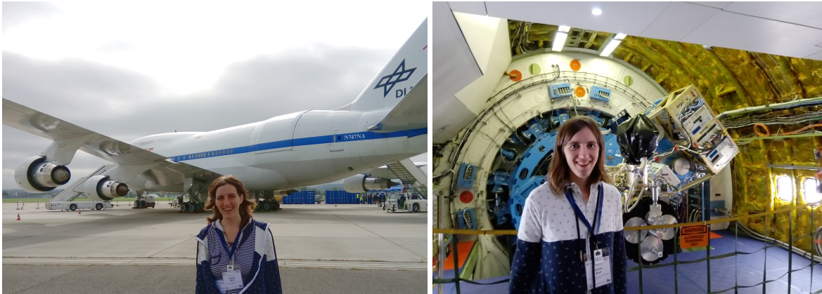
Figure A.4: SOFIA together with the author from out- ( left ) and inside ( right ). The HAWC+ detector is mounted (right panel). The telescope sits -airtight- behind two port-side cavity doors inside the airplane fuselage (just behind the science instrument). The telescope door remains open during the flight. The images are taken in Stuttgart in September 2019.
