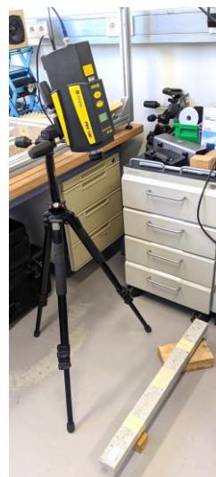
Figure 6. An overall view of the test setup showing the laser vibrometer pointing at the mid-span of the beam (similar to the test setup in [12]).
