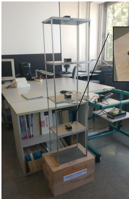
Figure 2. Experimental setup with the laboratory test structure instrumented with the wireless SHM system.
