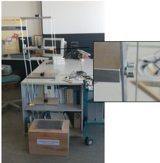
Figure 4. The damaged test structure and the location of the damage.
