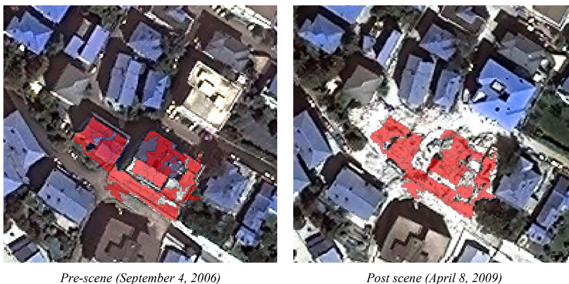
Figure 10. Detection of changes in the roof of buildings after applying SVM ( DigitalGlobe, 2006 & 2009 ).
