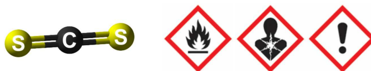
Figure 3.1: Molecular structure, and chemical hazard pictograms of \text{CS}_2 . The linear molecule consisting of one carbon and two sulfur atoms is highly flammable, poses several health risks and is toxic to aquatic life.
