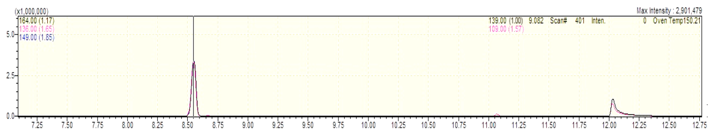
Figure 2. Method validation: GC-MS, extracted ion chromatogram, with the peak for TQ detected in NS oil No. 3 after 8.55 min and IS-M after 12.05 min.
