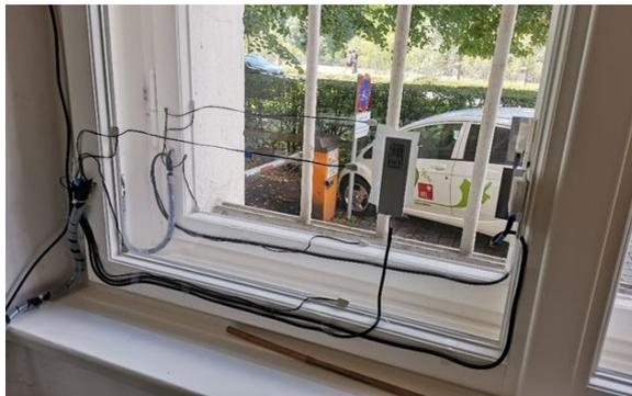
Figure 6: top: one of the examined case-study buildings; bottom: Monitoring equipment in a vacuum-glass equipped casement window (source: the authors)
