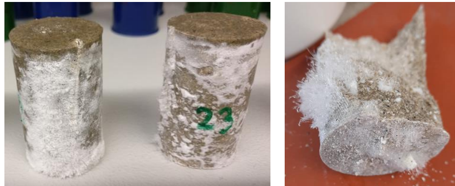
Figure 9. Salt efflorescence of the aluminum orthophosphate-based geopolymer binders.
