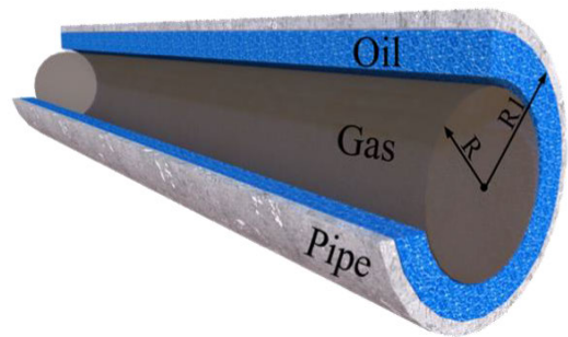
FIGURE 2. Two-phase annular flow pattern structure.
