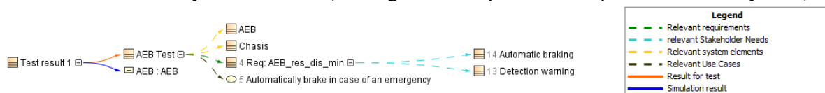
Figure 7: Traceability from a modeled test result to further elements of the system of objectives to support test interpretation [65]
