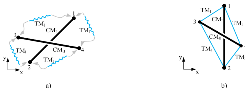
Figure 2: 2D tensegrity structure (compressed members: thick black lines, compliant tensioned members: thin blue lines); a) connectivity of the members; b) static equilibrium configuration in case of applying tensioned members TM_I with identical parameters.
