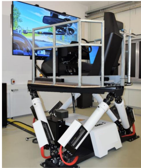
Figure 2: Dynamic driving simulator of the laboratory environment
