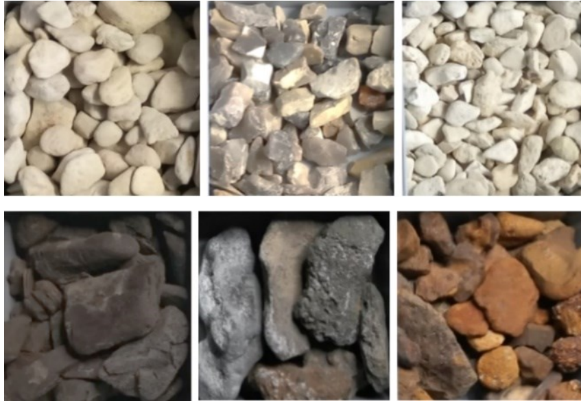
Figure 1: Examples of critical aggregates in concrete production (from left to right: opal sandstone, flint, chalk, coal, pyrite / marcasite, brown iron)
