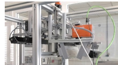
Figure 15: Demonstrator for the detection of rocks in the size range 8-32 mm using VIS-RGB camera and SWIR-HSI camera at GFE - Präzisionstechnik Schmalkalden GmbH
