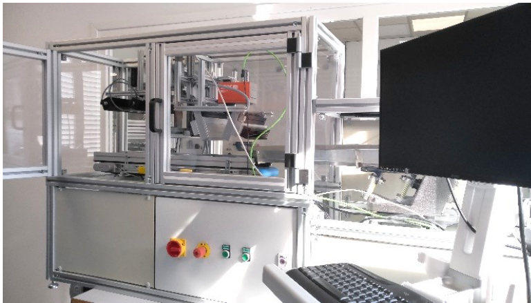
Figure 15: Demonstrator for the detection of rocks in the size range 8-32 mm using VIS-RGB camera and SWIR-HSI camera at GFE - Präzisionstechnik Schmalkalden GmbH
