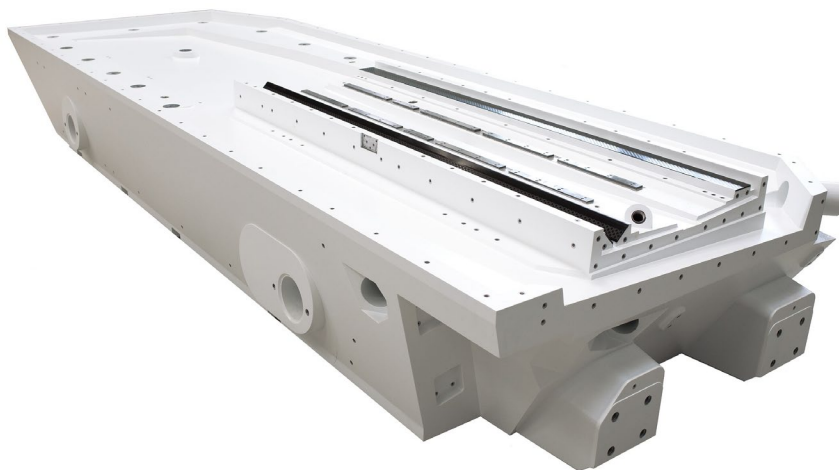
Figure 1: Machine frame part of a grinding machine made from polymer concrete with metal inlays and precision linear axis as a technology example [35]
