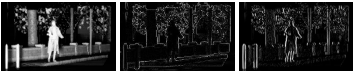
(a) Grayscale original image (b) Grayscale absolute contrast (c) Grayscale absolute gradient
