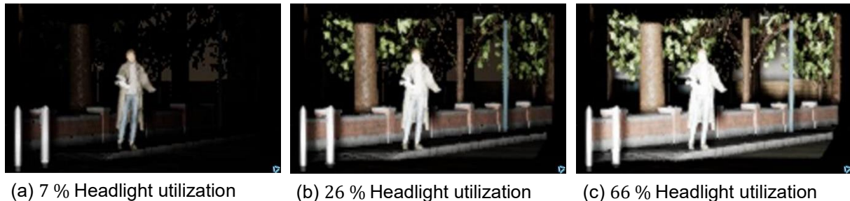
Figure 4: Camera image for three different headlight utilizations. All pixels are set to the same relative power value, so that the resulting intensity distribution is homogeneous.
