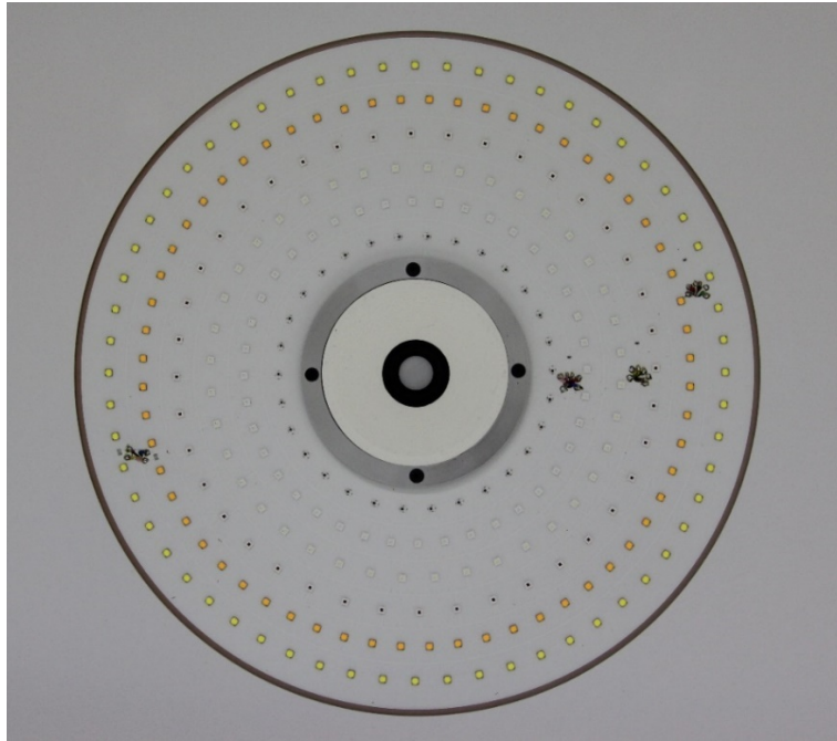
Figure 6: The front of the LED ring
