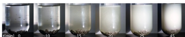
Figure 1. Reaction course of the iGMM, using calcium, (H)hmds and EtBr. The reaction starts with a slight gas evolution, followed by a turbidity, due to the formation of THF-insoluble \text{CaBr}_2 .
