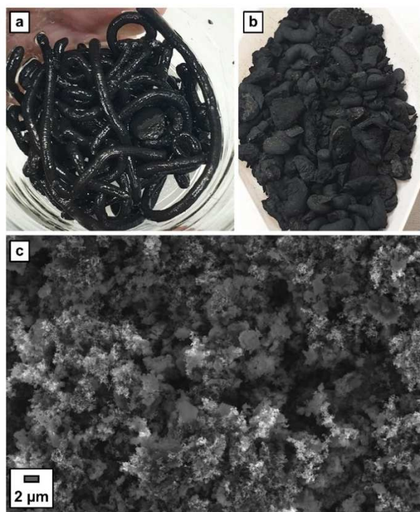
Figure 3. a) Composite material “worms” after extrusion from a syringe into the calcium chloride solution. b) Dried composite material after lyophilization and cutting into smaller particles. c) Scanning electron microscopy image obtained from the extruded and dried composite material. The small circular particles are the conductive agent particles that surround the polymeric active material.
