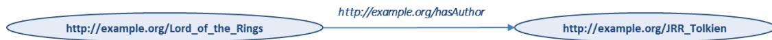
Figure 2.6: An RDF graph visualizing the relationship between a book and an author.
