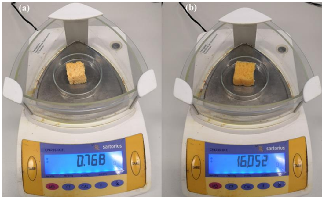
Figure 5-14 (a) and (b) Photographs showing the weights of superhydrophilic porous sponge before and after soaking saturated water.
