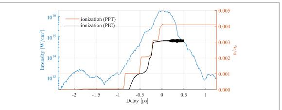
**Figure 2.** From the 3rd order autocorrelation of the chirped pump pulse the measured pulse duration is 600 fs. The pulse intensity is above the ionization threshold over a range of about 3 ps. The ionization fraction of the later presented PIC simulation are shown for comparison.
