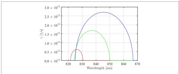
**Figure 4.** Growth rate obtained by numerical solution of the Raman dispersion relation. Parameters for the curves are: (a)  $I_{\rm P}=1\times10^{15}~{\rm W~cm^{-2}}, n=0.001~n_{\rm c}$  (red line), (b)  $I_{\rm P}=5\times10^{15}~{\rm W~cm^{-2}}, n=0.002~n_{\rm c}$  (green line), (c)  $I_{\rm P}=1\times10^{16}~{\rm W~cm^{-2}}, n=0.003~n_{\rm c}$  (blue line).
