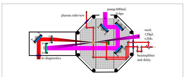
**Figure 1.** Experimental setup in the JETI vacuum chamber. The seed and side view beam paths passed additionally delay lines which is not shown here. The seed pulses are spectrally broadened in a gas filled hollow core fiber and subsequently compressed before they enter the setup as shown on the right.
