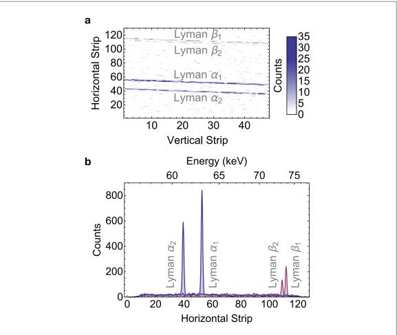
**Figure 2.** (a) Coincident x-ray spectrum as recorded by one of the FOCAL spectrometers. (b) Spectrum of the Lyman- $\alpha$  (blue curve) and  $-\beta$  (red curve) doublets of Au<sup>78+</sup> obtained by projections of the respective two-dimensional intensity distribution shown in (a).
