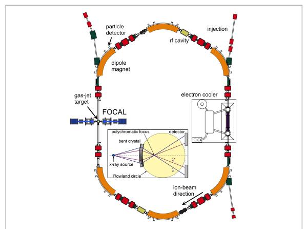
**Figure 1.** Schematic view of the ESR storage ring and the location of the FOCAL spectrometer at the gas-jet target. In the upper left dipole magnet a particle detector recording down-charged ions is used to apply a coincidence condition on the x-ray spectra. The inset shows a schematic view of the FOCAL crystal optics layout.
