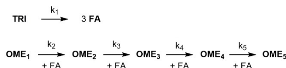
Scheme 2. Schematic representation of the relevant reactions in the OME synthesis via TRI and DMM.
