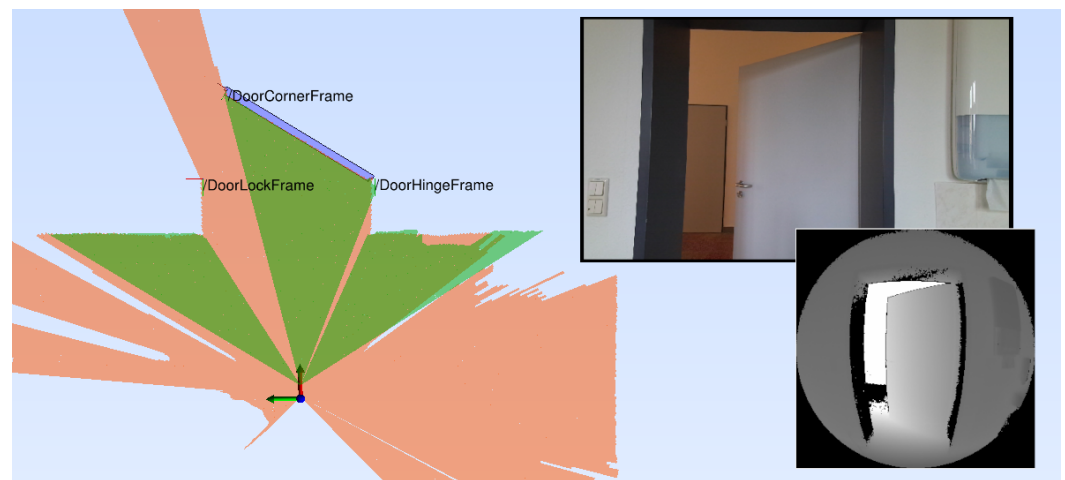
Figure 3. Exemplary sample of the doors dataset consisting of a SICK S300 range scan (orange), Kinect Azure color and depth image, and the annotation of the door's keypoints. The green range scan is a horizontal line from the depth image. The blue polygon is the model of the door panel with its known geometric parameters.
