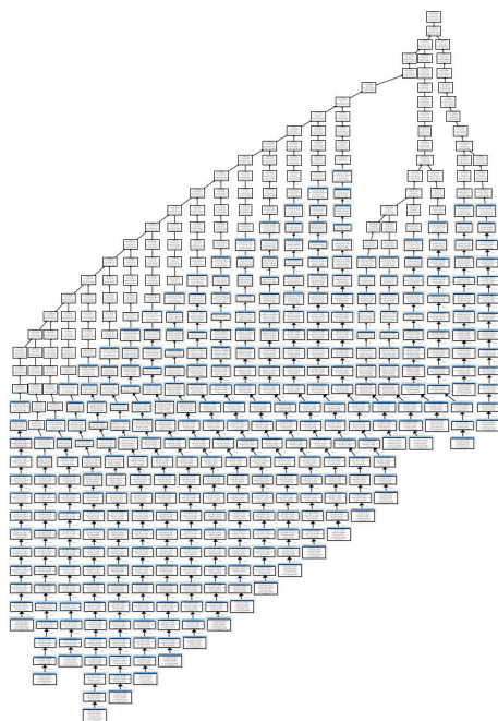
Figure 2.3: Overview over a query generated by a dashboard tool. Every branch is a distinct query. Graph generated using Actian Vector.
