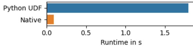
Figure 2.4: UDF vs. native performance for modulo operation on 8 million tuples
