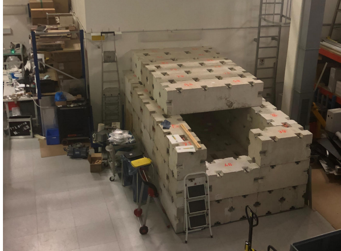
Figure 5.8.: Detection bunker installed at CALA behind a 5.6 m radiation shielding wall of concrete. The bunker is connected to the CALA target area by a 10 cm diameter tunnel.
