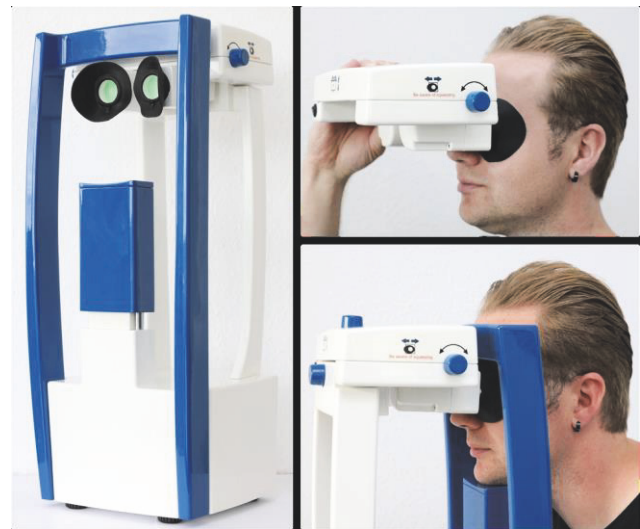
Figure 1: PEP-2000 diagnostic device as stationary and hand-held unit. (Source: ICM e.V.)
