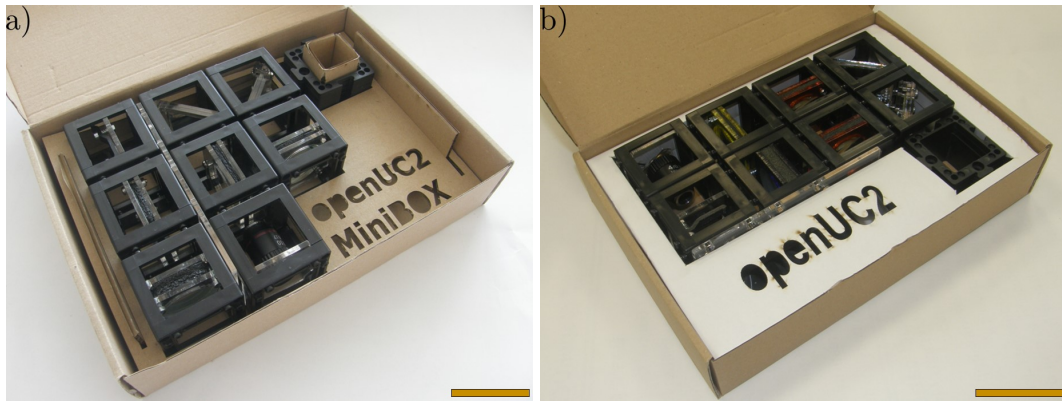
FIGURE 4.6: MiniBOX prototypes. a) Early prototype without distinction between the lenses. b) Final prototype in proposed packaging. Scale bars: 50 mm.
