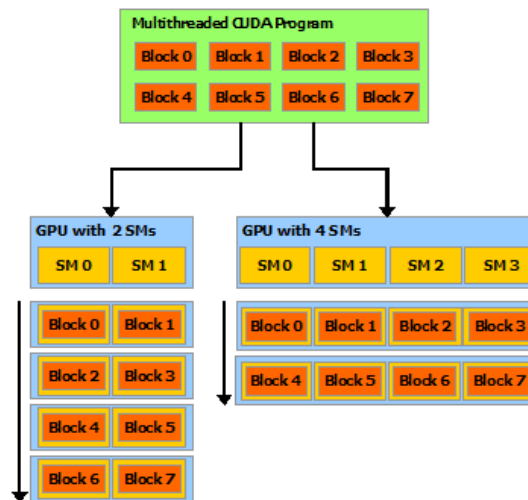
Figure 2-9 - left: Automatic Scalability. SM = Streaming Multiprocessor: Source: [19]
