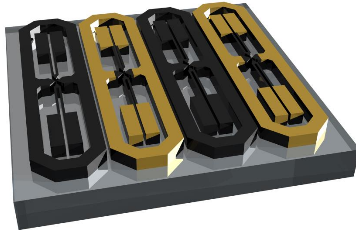
Figure 1. Layout of the four gradiometers on one and the same SrTiO 3 substrate. Black parts refer to pristine parts of the YBCO thin film, gold ones to YBCO with embedded Au nanoparticles.
