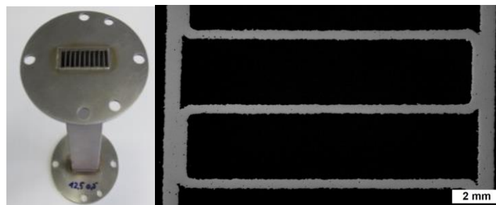
Figure 3. Test specimen and metallographic examination of test specimen with density >99\% .
