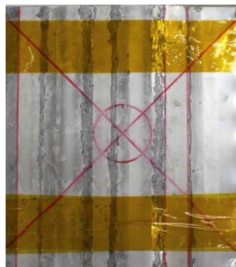
Figure 2. One-layer soldered 25 \times 25 \text{ cm}^2 superconducting sheet.
