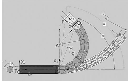
**Figure 7.** Model of probe under ante flex-retroflex
