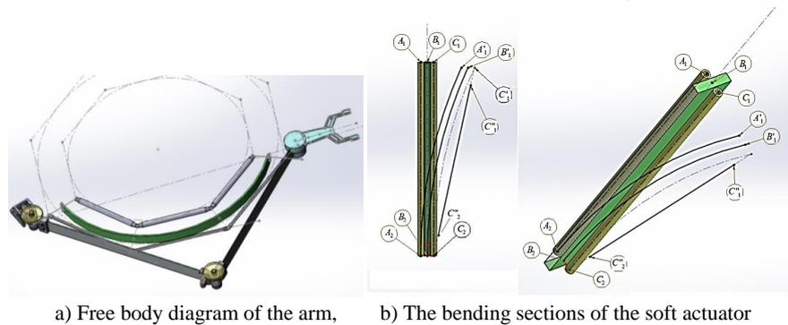
Figure 4. Design of the arm
