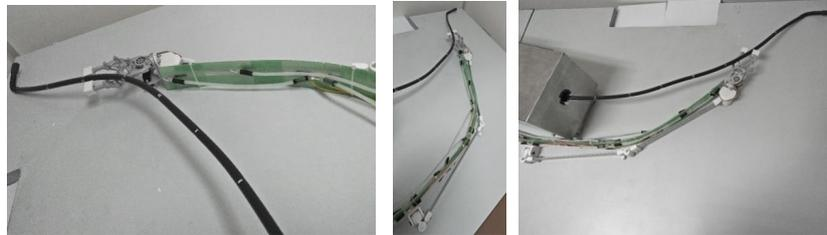
Figure 3. The flexible arm with soft actuators
