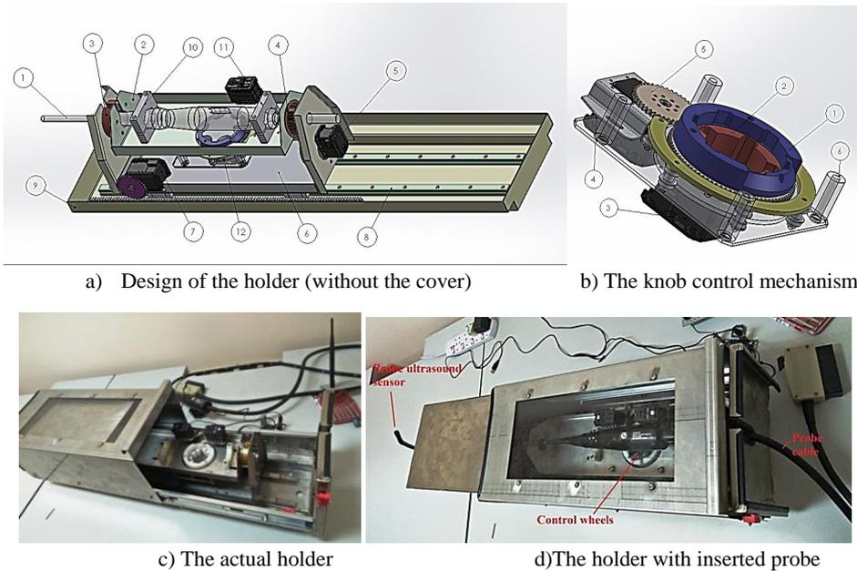
**Figure 2.** The holder mechanism and the fabricated prototype
