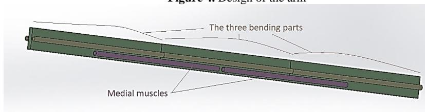
Figure 5. The overall soft actuator
