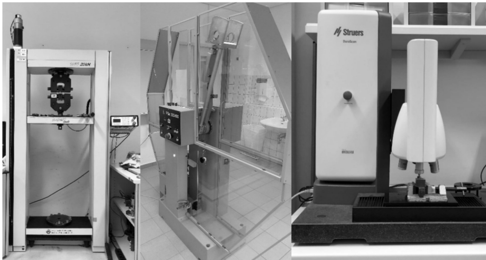
Figure 5. Testing equipment for mechanical properties; left: universal testing machine Zwick 1455, middle: WPM PSd 300/150, right: Struers DuraScan 70.
