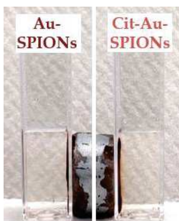
Figure A3. Magnetic separation of Au-SPIONs and Cit-Au-SPIONs after 8 h showed clear supernatants, which indicated that the gold was reduced onto the SPION cores instead of forming unattached nanosized gold that would appear red in the supernatant.
