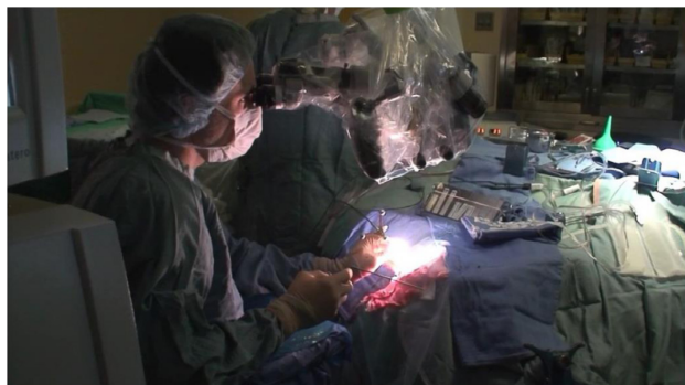
Fig. 13 Raman handheld probe being used in the operating room at the Montreal neurological Institute and Hospital by neurosurgeon Dr. Kevin Petrecca. The sources of ambient light can be observed including the microscope white-light, operating room overhead lights, and LCD screens (Reprinted with permission of JBO). 230
