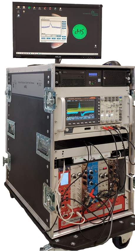
FIGURE 5.5: Photo of the developed electronic rack. The flight case includes a NIM crate with data acquisition modules, computer, oscilloscope, bias.
