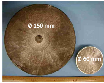
Figure 2.15: Photograph of two Gd-Ba-Cu-O bulk discs with diameter of 150 mm and 60 mm grown using oxygen controlled melt growth (OCMG) by Nippon Steel ® [91, 92].
