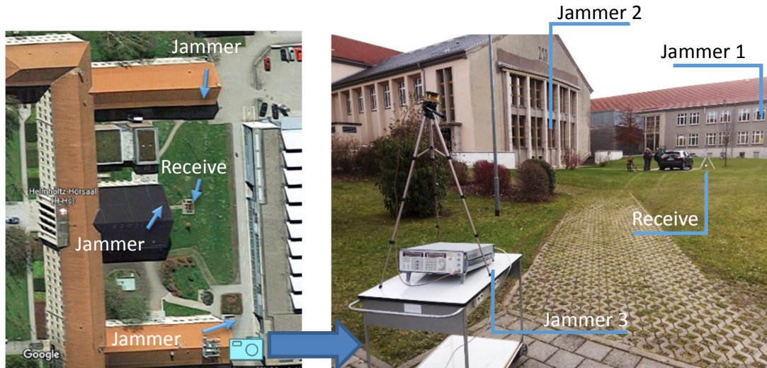
Figure 6.12: Top-view (left) and side-view (right) of the setup of the “measurement campaign Ilmenau 3”, with antenna placed either on a tripod or on the car roof. The test was performed in a 75 m x 30 m yard surrounded by buildings. Three jamming sources at three different directions were used.
