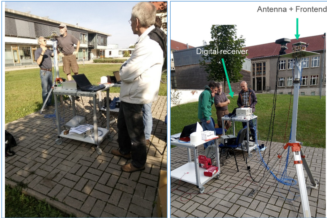
Figure 6.3: Measurement-setup in the measurement campaign Ilmenau 2, with the antenna system mounted on a tripod.
