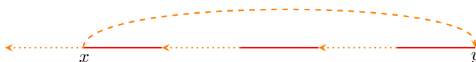
■ Figure 5 Red solid lines represent edges in M . Edge xy is not added to a Directed Semi-Matching because there does not exist a directed path starting from xy and not visiting x . The other orange dotted lines represent edges stored in Directed Semi-Matchings in previous iterations.
