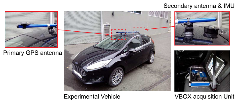
FIGURE 3.6: Experimental vehicle used to verify the virtual vehicle model implemented in IPG-CarMaker [6].
