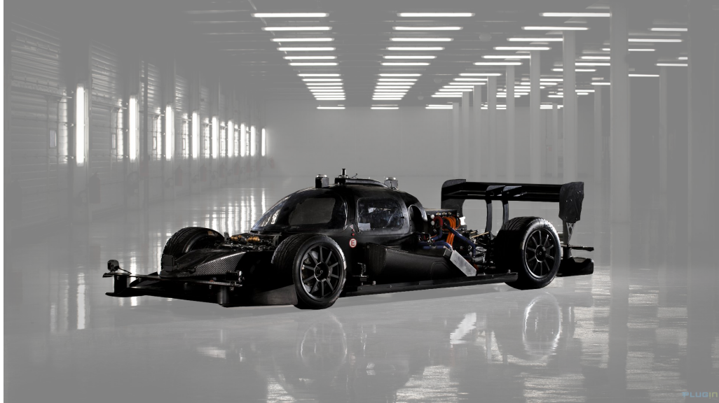
FIGURE 2.8: “DevBOT”, first autonomous race car developed by ARRIVAL and ROBORACE. This Multi-Actuated Ground Vehicle is equipped with four independent electric motors, independent front and rear brake-pressure lines and steering control. LiDARS, cameras, and a high-accuracy two-antenna GPS system complete the vehicle perception and positioning features.
