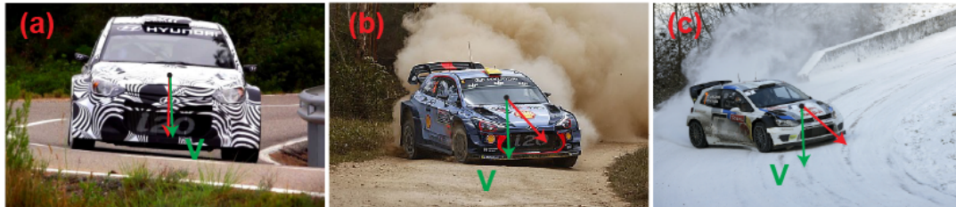
FIGURE 2.4: (a) Turning on tarmac (low body slip), (b) Turning on gravel (High body slip), (c) Turning on snow (High body slip).
