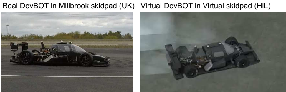
FIGURE 4.11: Real and virtual testing environments. The core development work was predominantly carried out in the virtual environment.
