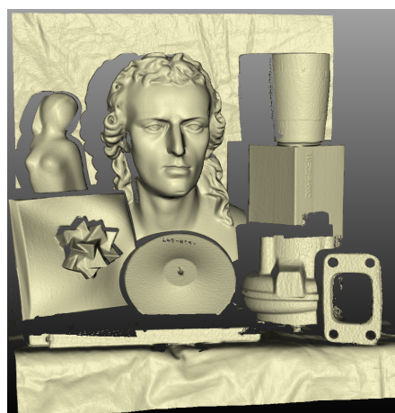
Figure 10. Ground truth 3D model calculated from 400 image pairs.
