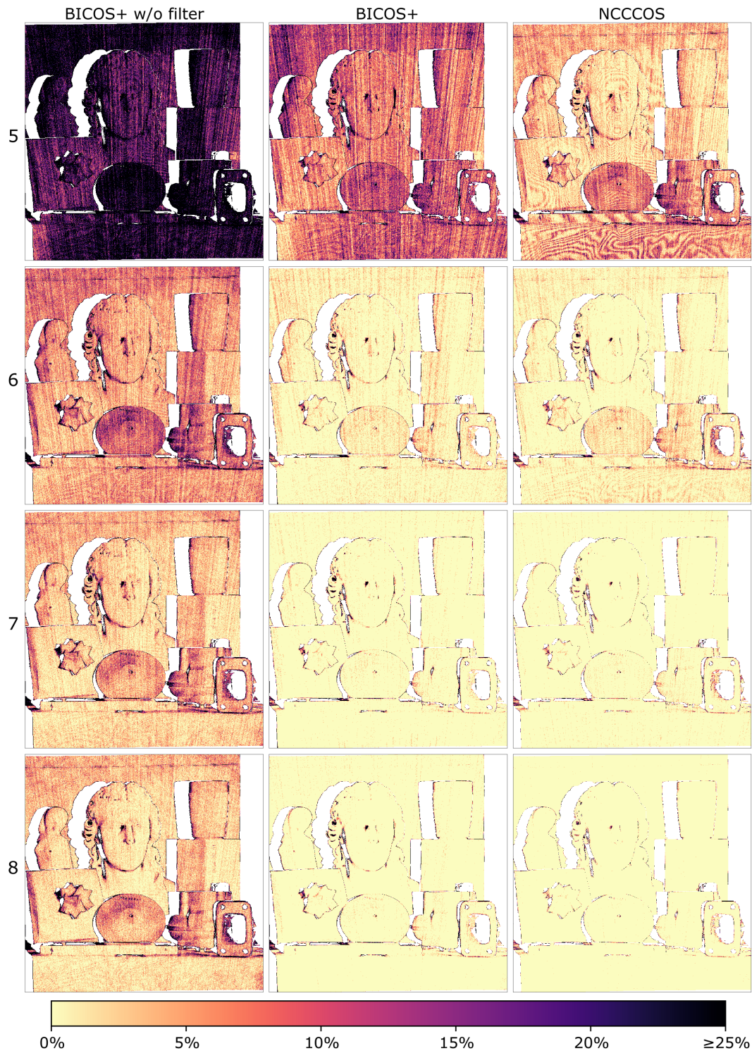
Figure 13. Percentage of wrong or missing correspondences (out of 39 data sets). Top to bottom: sequence lengths 5, 6, 7 and 8. Left to right: BICOS+ without median filter, BICOS+ (with median filter) and NCCCOS.
