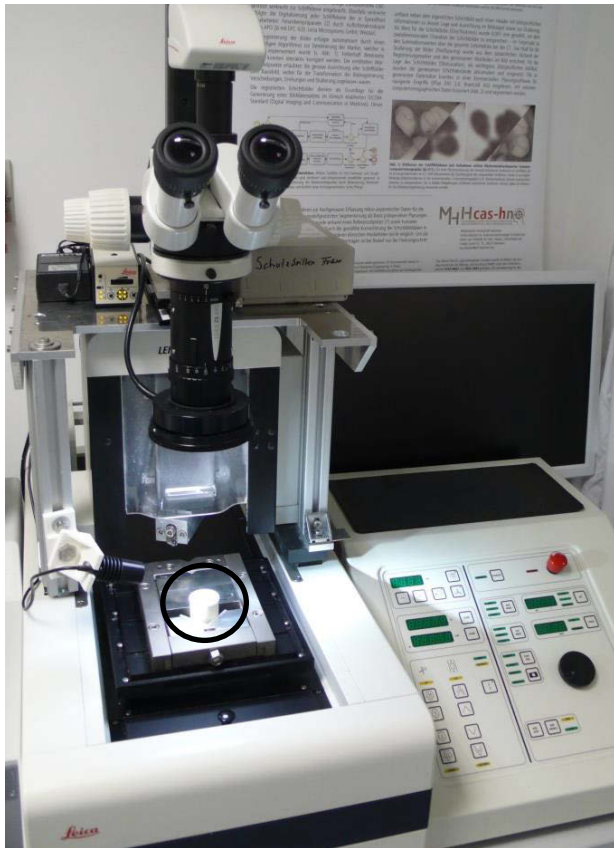
Figure 1: Automated microgrinding setup. Microscope with camera is mounted on top of the lifting head of the milling cutter. A sample (black circle) is clamped within the microtome. The control unit is shown on the right hand side of the microtome.
