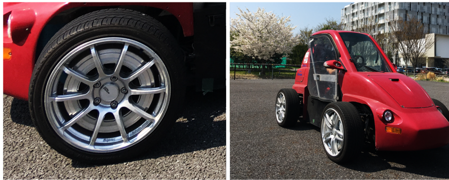
Fig. 6.3 Vehicle demonstrator with in-wheel electric motors: hub electric motor at front left wheel (left) and vehicle demonstrator at University of Tokyo testing track (right)
