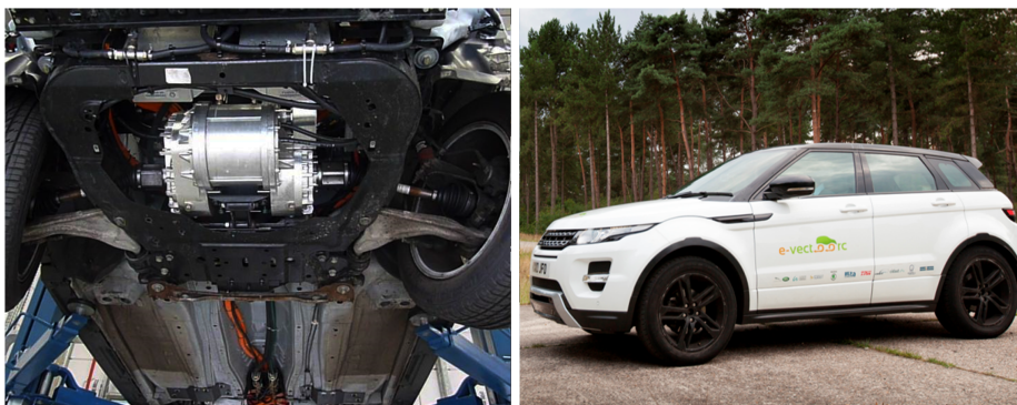
Fig. 6.1 Vehicle demonstrator with on-board electric motors: individual electric motors on the front axle (left) and vehicle demonstrator at Lommel Proving Ground (right)
