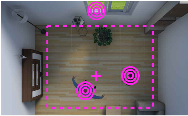
Fig. 5: The indoor scene. The sound is coming from the person, the radio and the open window, each source marked with concentric circles. The microphone position is marked by a cross. The user can walk in the area marked by the dashed rectangle on the floor.
