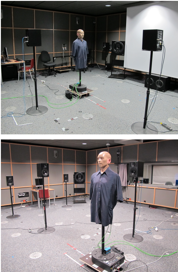
Fig. 1: The measurement setup in the listening laboratory.
