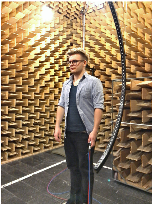
Fig. 3: HRTF measurement setup with a participant.
