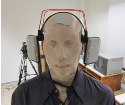
Fig. 5: Headphones AKG K1000 with a 45^\circ opening angle were placed on the HATS in order to enable a direct comparison of the binaural reproduction with the real loudspeaker reproduction.
