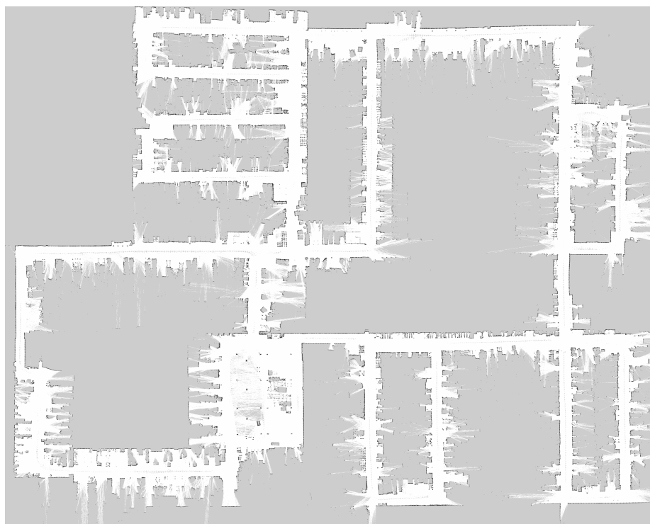
(a) The map generated using Graph-SLAM at 4 times of the real speed.
