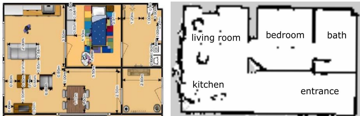
(a) The plan of the test area in project partner (b) The map generated using EMB-SLAM with two Focal Meditech BV. Kinects.
