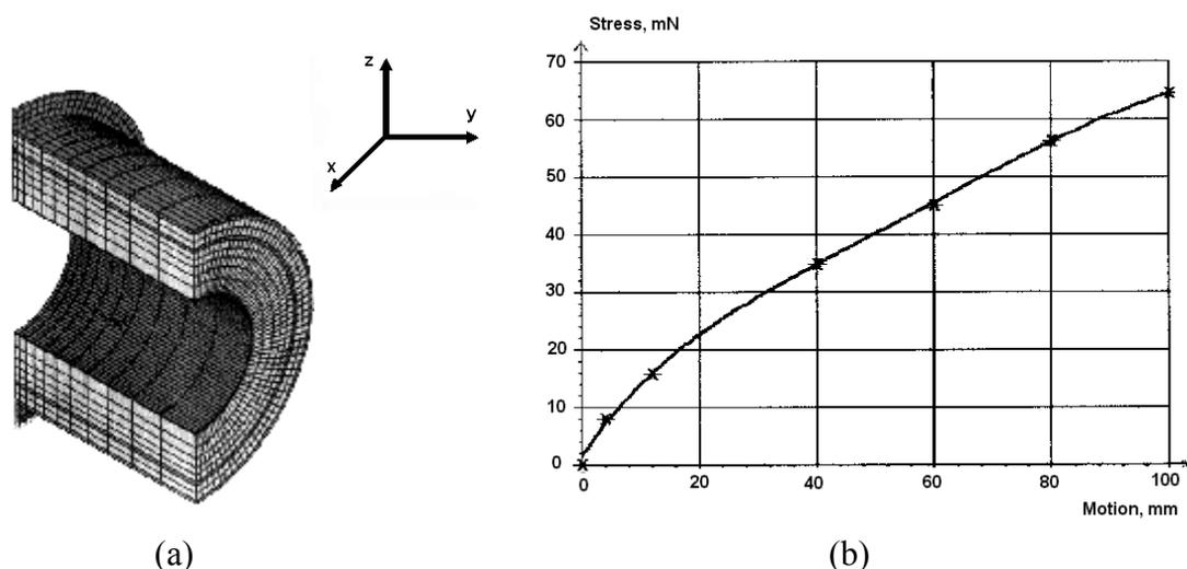
Fig.2. FE model of MCC (a) and calculation of stress in ring support (b).
