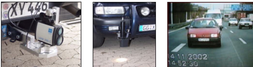
Rangefinder (left), Velocimeter (center) and video view (right) of the measuring car
