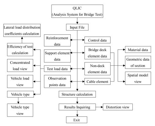
Fig.1 Diagram of system composition
