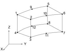
Fig.7 12-nodes solid element
