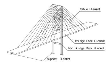
Fig.2. Diagram of position of elements
