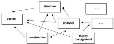
figure 2: relations between partial models reflect information needs
