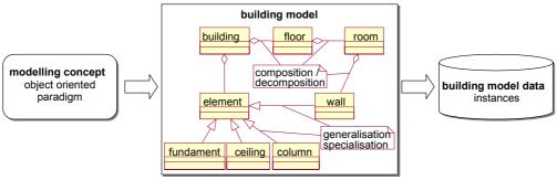
figure 1: object oriented modelling approach
